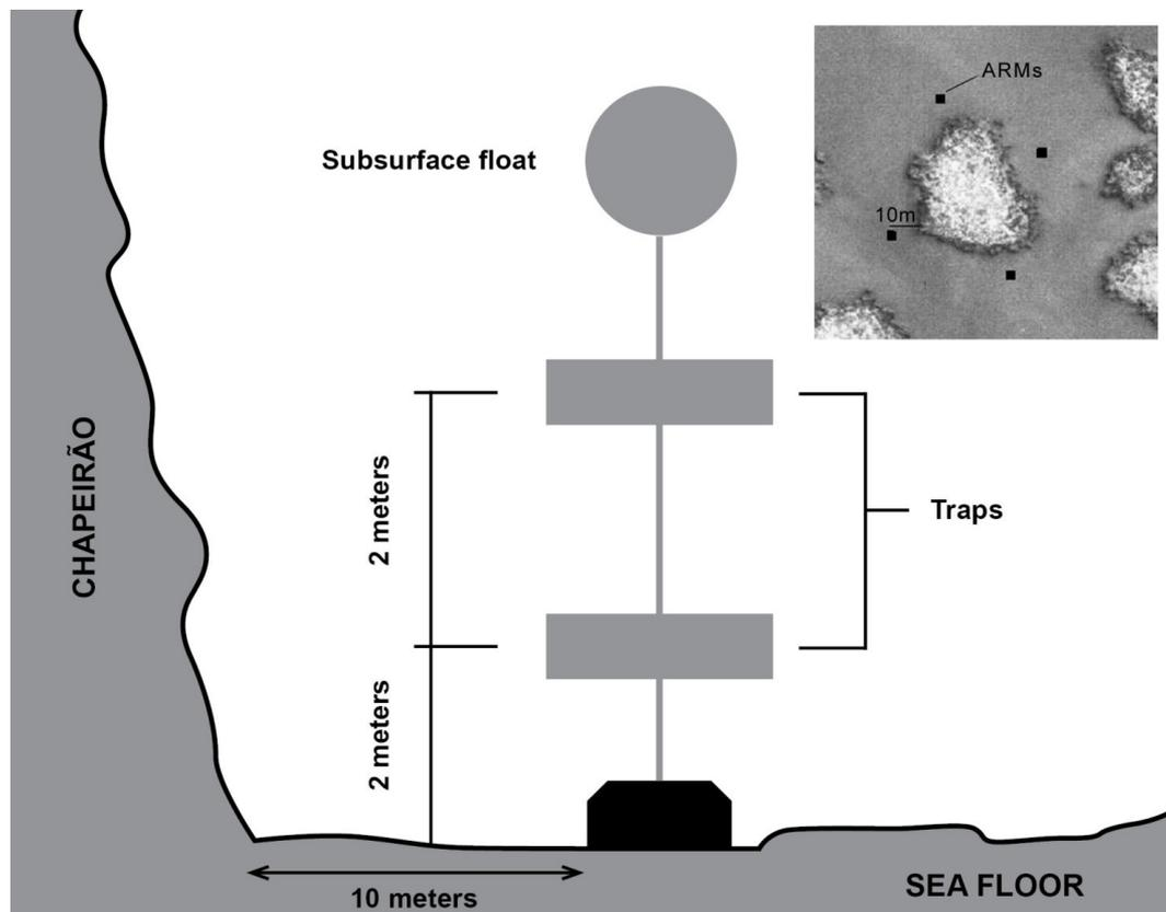
**Figure 2.** Illustration of the structure of the ARMs used and details of their placement around the stations.
